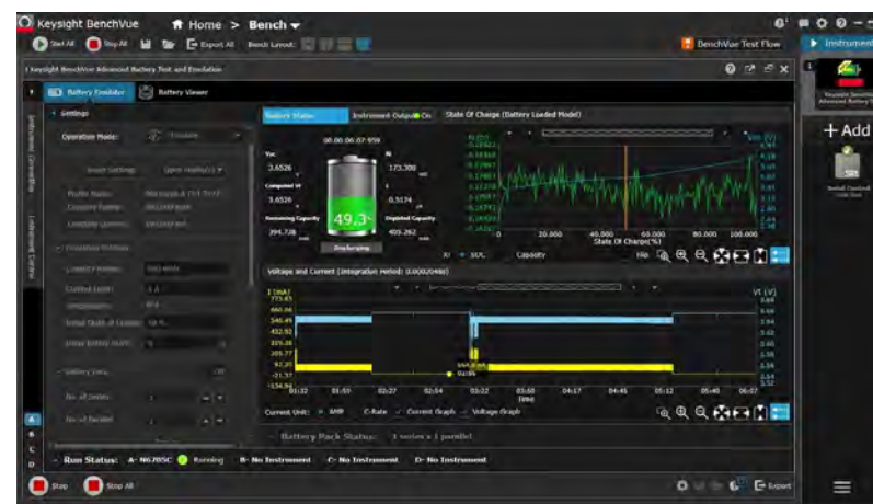
Figure 3. Battery emulation using BV9210B / 11B software
