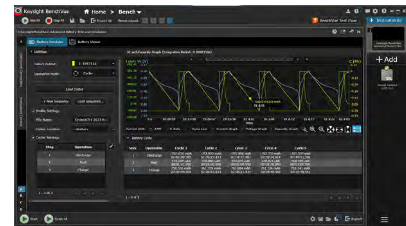
Figure 6. Battery cycling testing using BV9210B / 11B software
